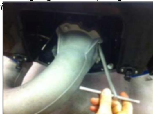
*To make sure that you have connected the top right screw properly, gently wiggle the elbow back and forth to ensure that you have tightened the screw correctly so that the elbow doesn't slide around.*
